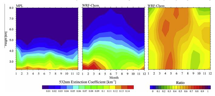
**Fig. 6.** Monthly vertical profiles of aerosol extinction coefficients at 532 nm for 2007–2011 from the MPL retrievals (right panel) and the corresponding WRF-Chem simulation (middle panel), and the dust contribution (dust extinction coefficient /total aerosols extinction coefficient) from the WRF-Chem simulation (right panel).
