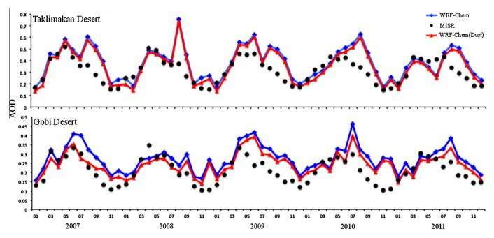
Fig. 3. Monthly total AOD over the TD and GD from the MISR retrievals (black dots) and the WRF-Chem simulations (solid lines) for 2007–2011. Both total AOD (blue line) and dust AOD (red line) from the simulations are shown.
